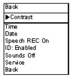
The display can be darkened or lightened by pressing the yellow Up or Down button. Press the green Select button to return to the Set Up Menu.
